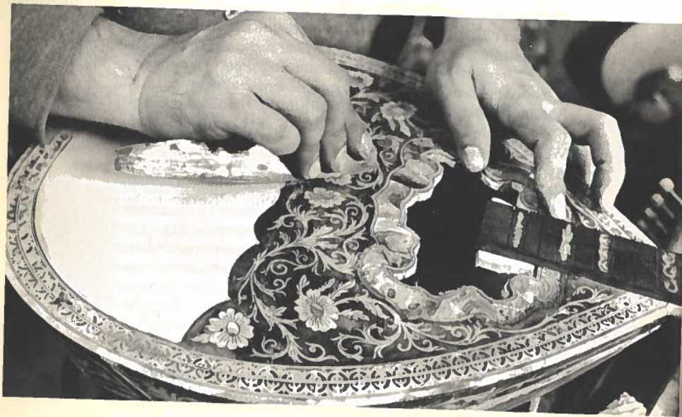
Karolos Tsakirian sands mother-of-pearl inlay on a Greek bouzouki top. photo: Martha Cooper
